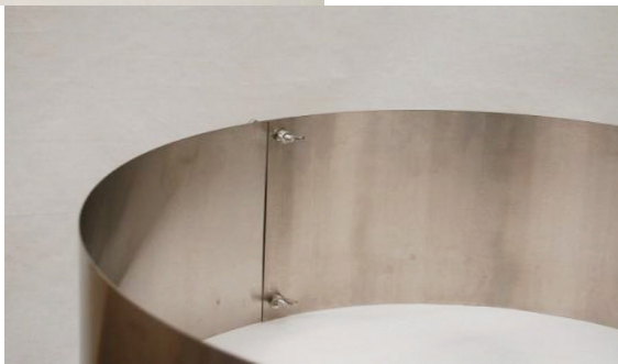
18.5 Inch Assembly (note overlap which decreases diameter):
